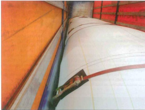
Büscheroff's new design of 40ft, multi-layer, flexitank for use in trailers and containers comprises seven compartments
